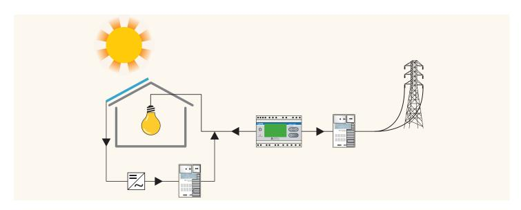
eVison allows you to visualize with a simple click your actual, day, week, month and annual Energy consumption. Understand how and how much you are spending has never been so simple. eVision is perfectly adaptable to a solar plant. It will indicate the quantity of generated and consumed Energy calculating automatically the cost or the earning of your house.
